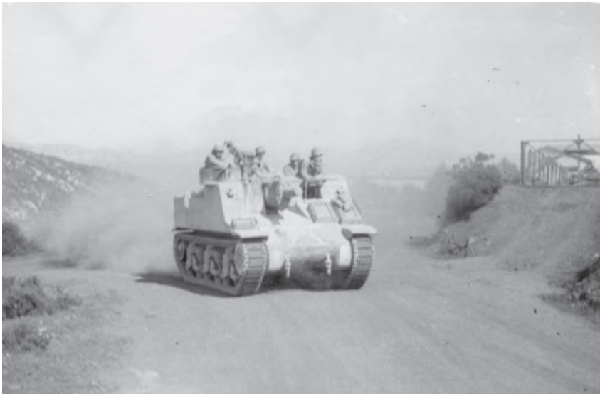
Figure 10: M-7 "Priest" self-propelled howitzer assigned to the 16th Infantry's cannon company near Tébessa, Algeria, on the Tunisian border. Soldier photo, MRC
