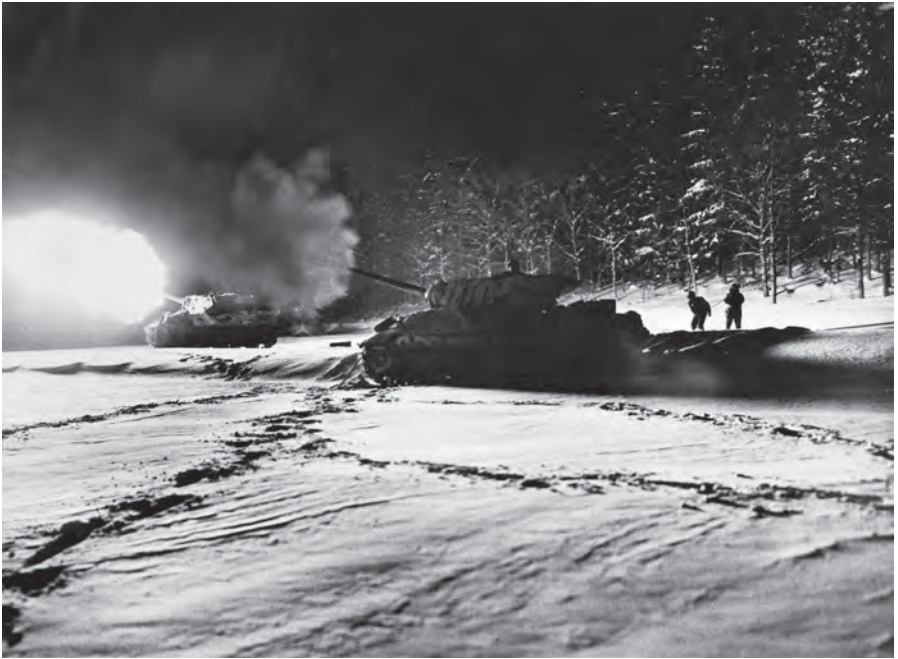
Figure 38: M-10 Tank Destroyers firing as artillery on January 26, 1945. The M-10 in the foreground is using propellant designed to reduce the flash. The one in the background is firing with far less stealthy propellant. Signal Corps photo, Fort Riley Museum Complex
