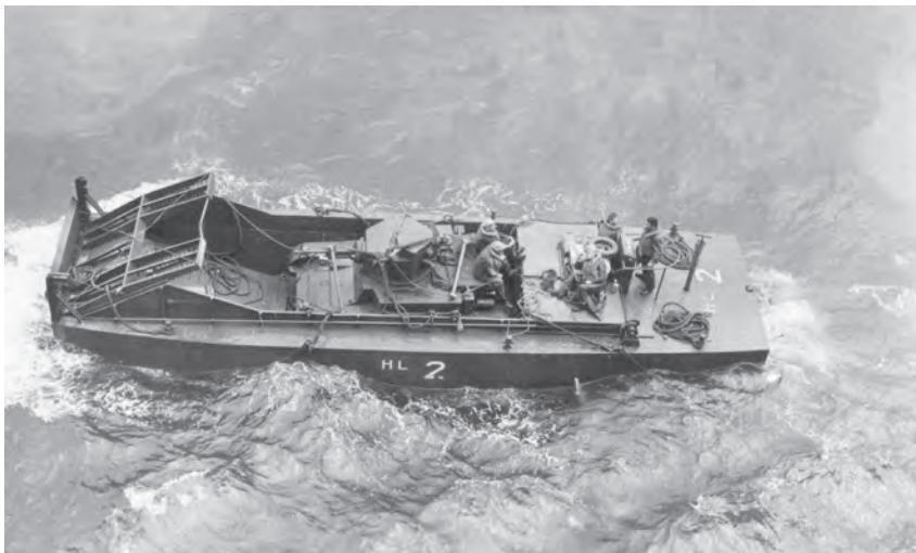
Figure 3: An early amphibious craft seen from the Wakefield . Note the rails on the ramp for unloading vehicles, in this case a light tank. Soldier photo, MRC
